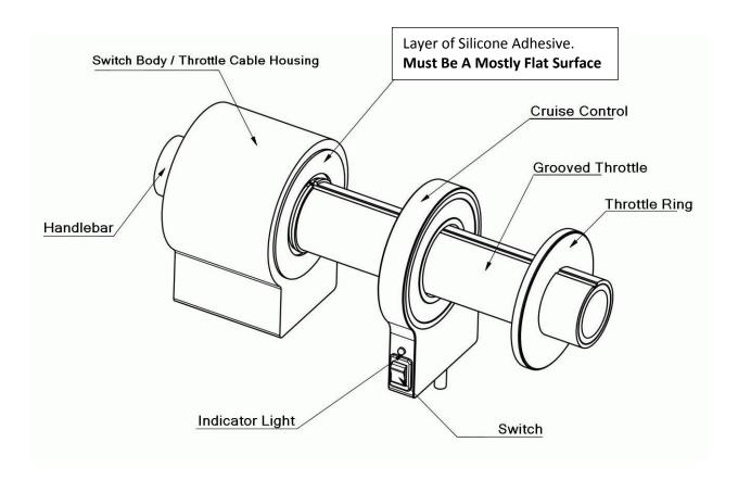
The cruise control unit must be attached (glued) to the motorcycle's Switch Body / Throttle Cable Housing with silicone adhesive.
