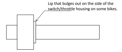
This style of switch/throttle housing does not have enough of a flat side for the cruise control unit to adhere to.
